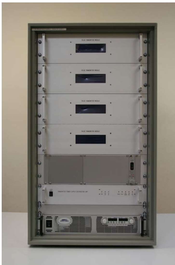
Pulse Transmitter System Comprised of Four Pulse Transmitter Modules
